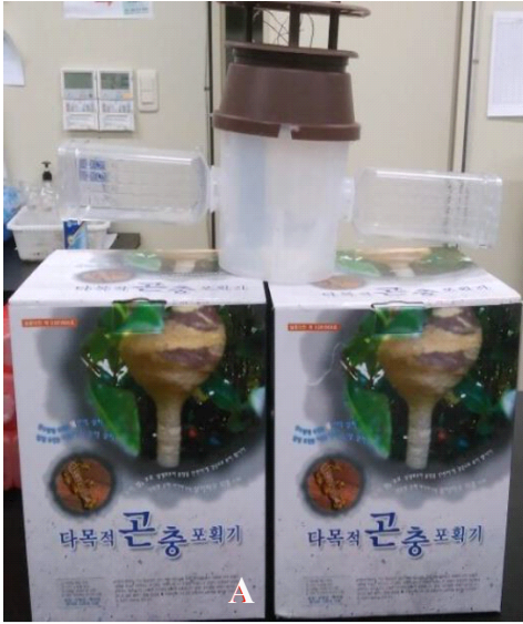
Fig. 3. Commercial traps used to collect Vespa including V. velutina . (A) An assembled trap, along with commodity packing box, manufactured by DAMOK Ecological Technology. (B) Entrance part, (C) Cylinder-shaped attractant container (Ø 13.5 cm), (D) Collecting bottle (56 holes, Ø 6 mm) and (E) Shield part for the prevention of captured Vespa to access to attractant solution.
